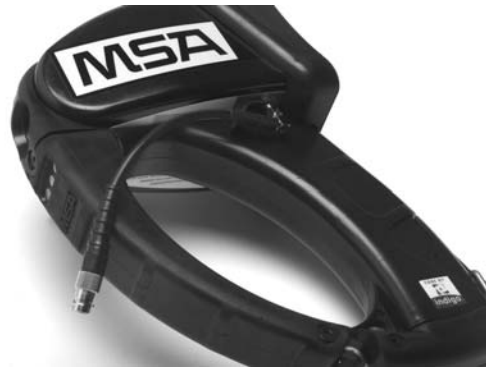
Figure 5. TIC with SMA to BNC Connector
